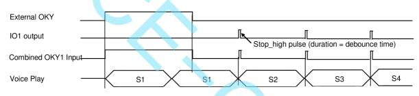
% Originally the duration of Stop\_high pulse is 172ms at 6kHz, but the high signal will trigger voice and turn low after debounce.
